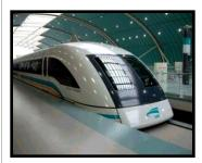
The Maglev train in Shanghai is the first of its kind in the world; made of breakthrough German technology, the Magnetic Levitation (Maglev) Train is the new state-of-the-art mode of transportation in Shanghai. Using no wheels, the train floats on an electromagnetic cushion, which is propelled along a guide way at incredible speeds. Meandering for 33 kilometers
